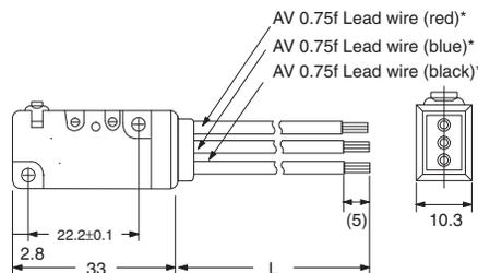
\* UL/CSA approved models have AWG20 UL1015 approved wiring.
