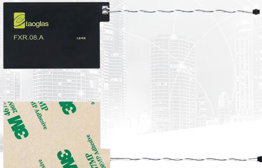
The FXR.08.52.0075X.A is a rectangular, flexible, NFC (Near Field Communications) antenna for use in mobile devices and other applications such as keycards, payment systems, and boarding passes. The design provides a flexible NFC antenna with 75mm twisted pair 28AWG cable that can be adhered to the plastic enclosure of the device for ease of installation and work with specific 13.56MHz RFID and NFC chips which need to connect via JST ACH connector.
