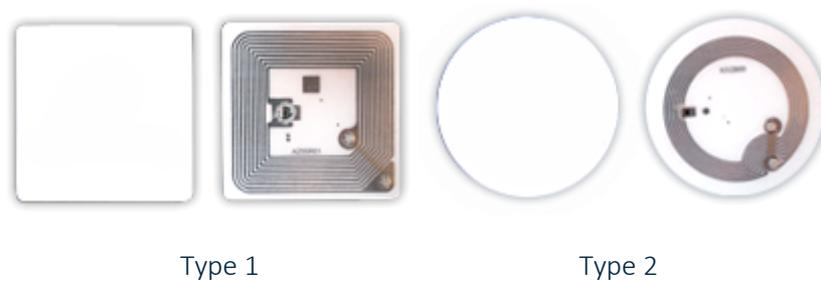
Type 1 tag is based on ISO/IEC 14443A standard and has 512 bytes of memory.
