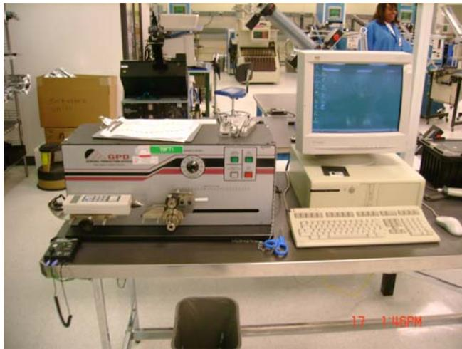
Figure 16 Peel-Back Force Test (PBFT) System.
