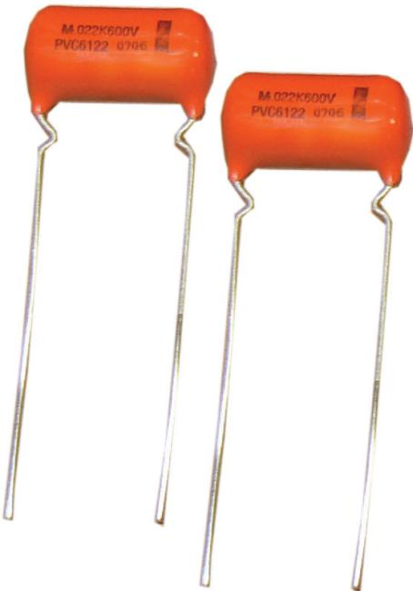
The Type PVC is a sturdy film and extended foil construction ideal for bypass and coupling applications. Extended foil construction is as good as it gets for low DF and high current applications. The PVC is encapsulated in a rugged, flame retardant, epoxy coating with the leads crimped to provide secure seating on printed circuit boards.
